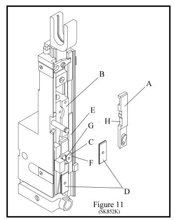
3. In conjunction with the grip release slide (Index E), it controls the movement of the bender bar latch (Index F) that opens and closes the grip (Index G).
