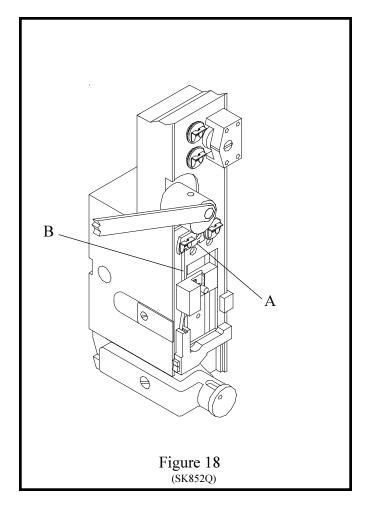
If the corners of the top surface of the supporter are too sharp, or nicked, the corners of the stitch crown will fracture. If operating properly the supporter should function as follows:
