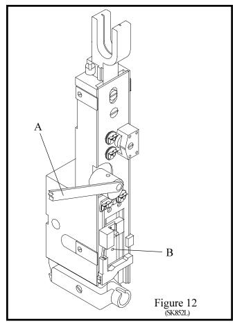
the driver riding on top of the formed stitch. When the bender bar is stopped against the work material, the driver continues downward to exert pressure on the crown of the stitch, driving it through the work material.
