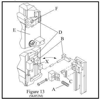
When the face plate (Index E) is adjusted (See "Changing Work Thickness", page 6) a pivotal action (at point F) changes the position of the grip slide. When the face plate is raised, it moves the grip release slide down. The gripper can then remain closed longer, on the down stroke, feeding more wire for the stitch. When the face plate is lowered, it moves the grip release slide up. The gripper will open sooner on the down stroke, feeding less wire for the stitch.
